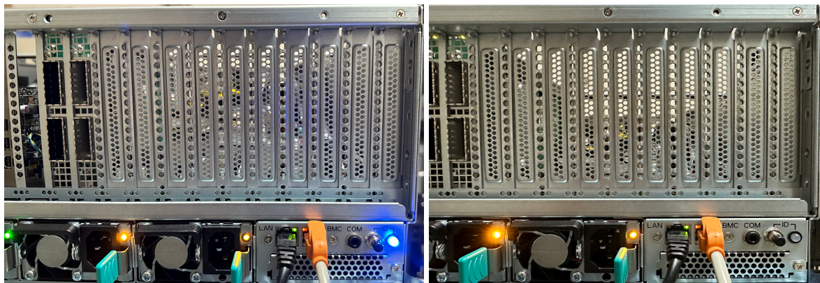
Figure 25. UID Light Blinks Twice Before System Power-On
