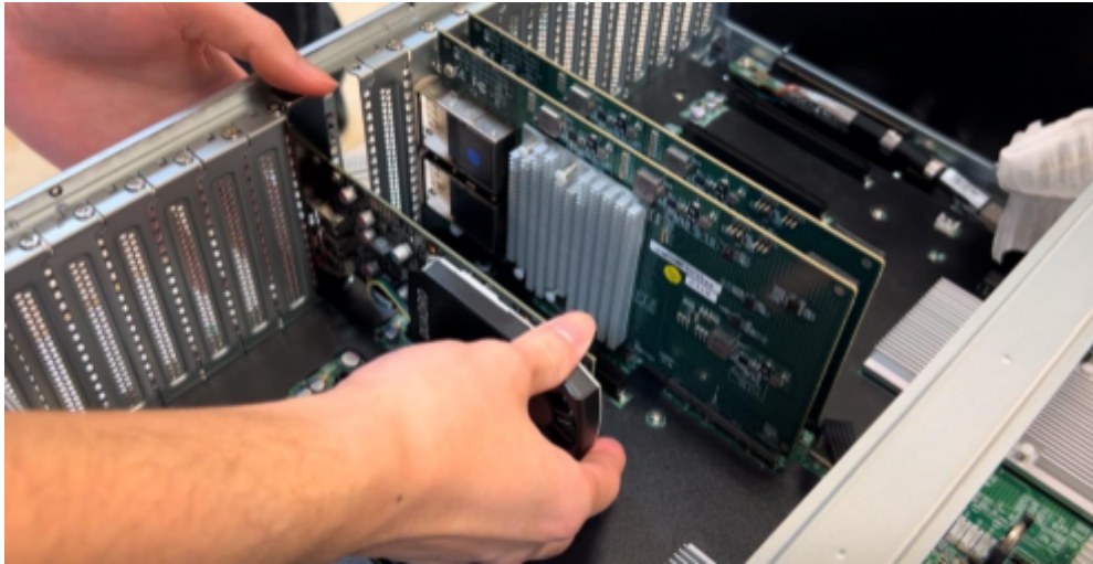
Figure 36. Installing a Single-Width Device into the PCIe Slot
