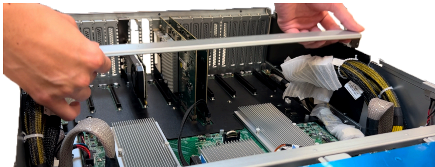
Figure 30. Removing the Stabilization Plate for Internal Component Access
