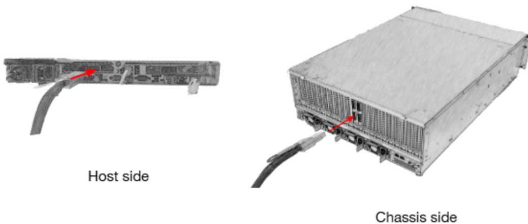
Figure 49. Host and Chassis Connections Using CDFP Cables
